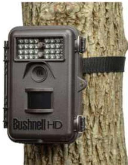
Figure 3. A Bushnell Trophy Cam Trophy HD camera trap used in the St. Edward Park study, attached to tree. The camera uses a passive infra-red sensor to detect motion, and a “low glow” infra-red flash to take pictures at night without disturbing the subject. Photo by Nik Burns.
